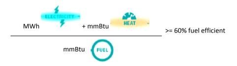
The values needed for the calculations above can be measured and the formulas can be applied in topping cycle systems.
