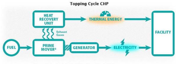
\*Internal Combustion Engine/Gas Turbine/Microturbine/Fuel Cell
