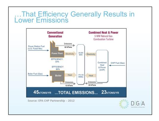
NB: CHP can produce electricity with  $\frac{1}{4}$  the emissions of conventional generation (450 to 600 lbs/MWh for NG-fired CHP vs. 2000 to 2200 lbs/MWh for coal).
